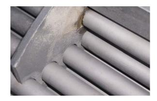
Partially ferromagnetic materials like Monel Alloy 2205, SA-789, nickel and thin ferromagnetic tubes materials include SA-268 or SS-439 can be tested by eddy current but with the saturation technique.
